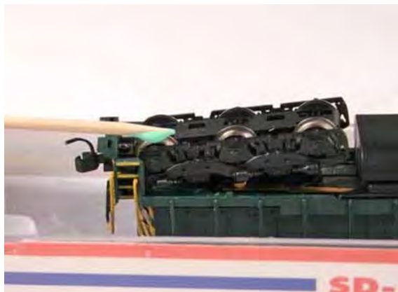
Installing BULLFROG SNOT, just touch it to the rotating wheel. "Yard speed" works well.
