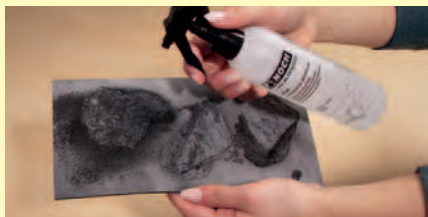
The rock former is prepared with a release agent made from water and detergent.
