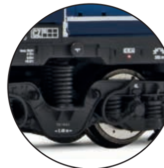
Fine detailed bogies with metal brake discs
