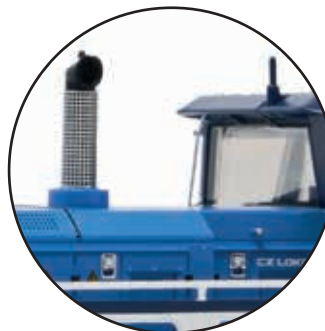
Exhaust pipe panelling made from photo-etched
