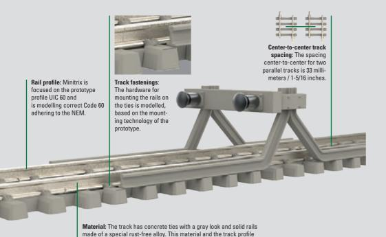
offer reliable contact for current transfer to wheels.
