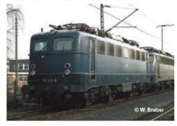
**Prototype**: German Federal Railroad (DB) standard design electric locomotive, road number 110 246-6. Cobalt blue basic paint scheme. Version with double lamps, plastic rain gutters above the end windows and cab doors, double forced air grills (DDL), undivided engine room windows with rubber gaskets, and end grab irons. The locomotive looks as it did around 1988
