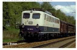
**Prototype**: German Federal Railroad (DB) standard design electric locomotive, road number 140 186-8. Ocean blue / ivory basic paint scheme. Version with double lamps, plastic rain gutters above the end windows and cab doors, Klatte design air grills, undivided engine room windows with rubber gaskets, and end grab irons. The locomotive looks as it did around 1979.
