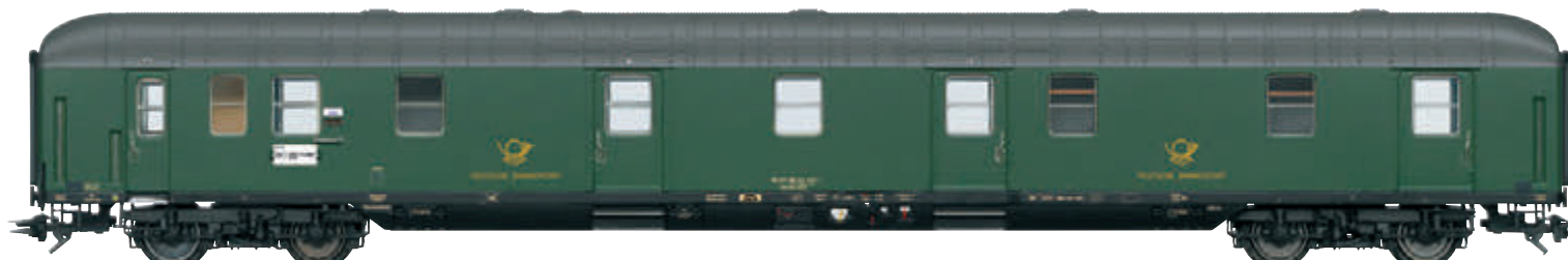
Prototypically equipped with Minden-Deutz (MD) heavy type 330 trucks including a type D 150 cardan axle generator
