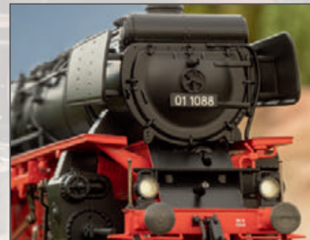
In the past, the streamlining covered the horizontally mounted Knorr feedwater heater as well as the flattened smoke box door.
